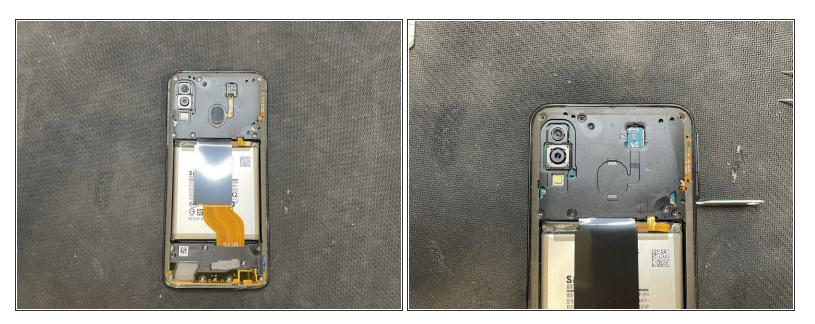
• Next, the 13 Phillips screws must be loosened so that the frame can be removed.
