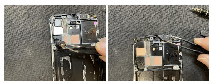
• Finally, the vibration motor and the earpiece have to be removed. You might need a bit of heat again to loosen the components.
