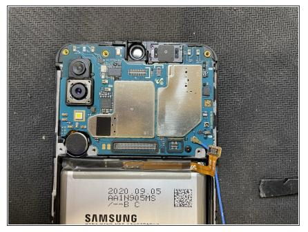
• Now the front camera has to be removed. This can be done with a spudger.
