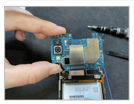
Now, both boards can be removed from the device. To do this, another screw must be removed from each of the boards.
