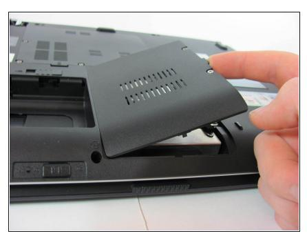
• To remove, lift up the panel's tab.
