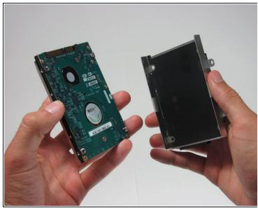
• Separate the hard drive from hard drive bracket to complete removal.
