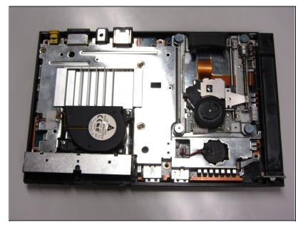
What you see in this picture is the electronic components found in the PS2. We are now going to remove the top metal casing found on top of the motherboard.
