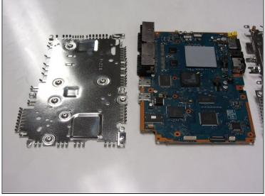
• Gently lift the metal plates from the top and the bottom of the motherboard.
