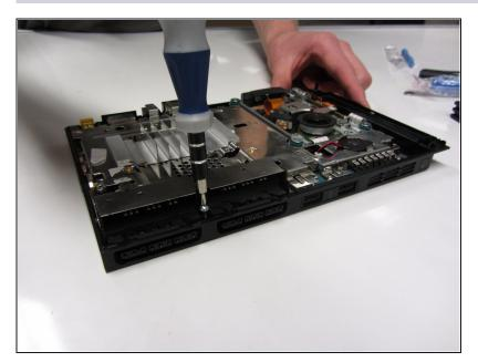
Locate the one 2.4mm screw that mounts the metal casing to the top of the motherboard and unscrew the screw with a Philips Screwdriver.
