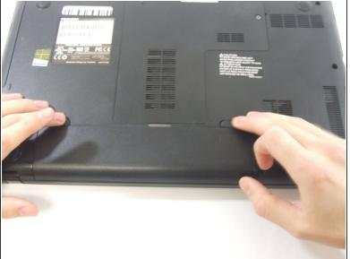
Slide the two lock tabs on the battery to the open position.
