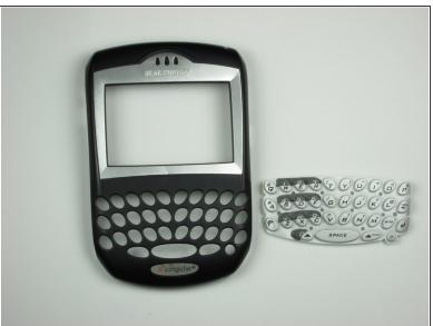
Peel off the rubber keypad buttons from the face plate.
