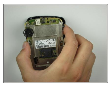
With one side loosened, simply lift the phone internals to separate from the front casing.
