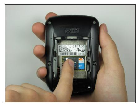
Slide the SIM card holder to the left to unlock the SIM card.
