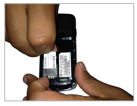
Remove the SIM card, by pushing down on the top of the SIM card and sliding it out from under the metal band.
