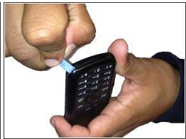
Use a wedge, or flat edged tool to separate the phone. Make sure to circle around the entire phone, especially the corners to pull it apart. This can be difficult. This may take several tries, so make sure to be persistent.
