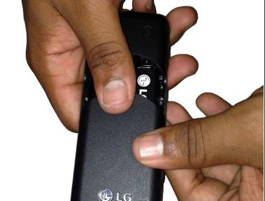
Remove battery back cover by applying pressure along the groove. The LG logo should be up right. Apply the pressure downwards to remove the cover.
