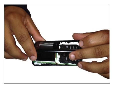
Separate and remove the two hard covers and the keypad.
