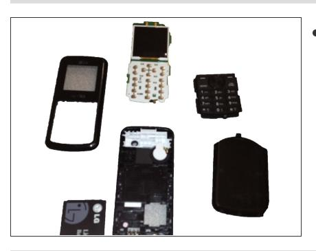
Once the phone is completely dissembled, you can replace the screen if it is cracked. You can also replace the keypad if the buttons do not work or if there are other issues with the keypad. Another common desire people have is to unlock the phone. In order to do this, you must replace the SIM card, which is explained in the steps above.
