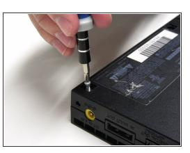
After all of the feet have been removed, Use a Phillips #1 screwdriver to remove the six 4.0mm screws from the base of the PS2.
