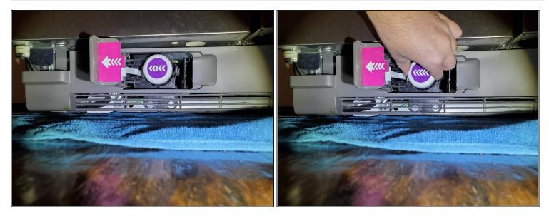
Open the door all the way and pull the filter out straight.
