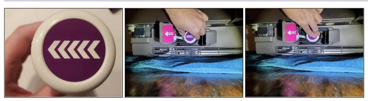
Point the arrow on the filter toward the left and slide it into the filter hole.
