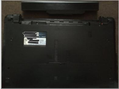
The battery can now be removed by sliding it out in the indicated direction.
