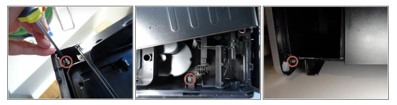
(i) Now the side part on the water tank side can be removed. It is still attached with three screws.
