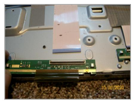
Close up of the display connector disconnected. Typical flip back the black bar and remove the ribbon cable,
