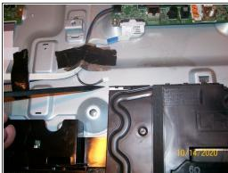
• The speakers are held into place with a tab at the top and 2 rubber pins in the back. Slide the tab into the slot and GENTLY push in the speakers, remember the glass display is in! Plug in the 2 connectors.
