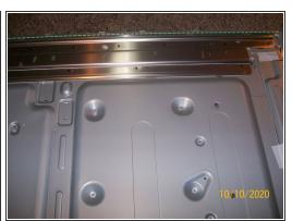
Here we can finally see the LED strips attached to the bottom of the frame. You can see the connectors. You can disconnect these now as we will attempt to remove them. They are held in place with thin, double-sided tape.
