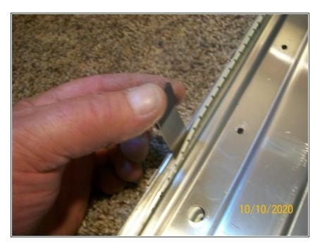
I started the removal process by inserting a thin metal tool between the strip and the frame. The tape came loose from the frame and stayed on the strip. I moved the tool down the length, prying very lightly. We'll be replacing these but I wanted to do the least amount of damage to them. I still need to read the part number off of them.
