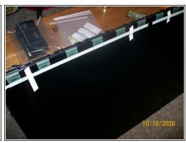
Back of set after rear cover removed. Bottom of TV at bottom of photo. The two speakers were removed by pulling up after disconnecting plug. Next is to remove the lower black panel that houses the power button and speaker mounts.
