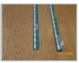
As you can clearly see, LEDs 2 and 4 on the bottom strip are burnt out. I verified this with a magnifying glass. This strip was from the right side that went dark. Next step is to order strips 6916L2318A and 6916L2319A and replace them and put this TV back together.
