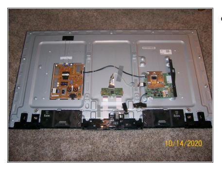
Here is the finished panel ready for testing. I kept the back off for now until I power up the unit. No telling if I forgot a cable. I stood the set up and put a couple of folded rags under each corner to hold it up off the floor so I can operate the power button. Now plug in the power cord and turn on the power.
