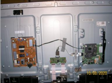
A few screws on the bottom and two plugs disconnected and the black bottom panel is removed. Now you can disconnect the display power connectors. There are 2 long green circuit boards (LCD drivers)strips at the bottom.
