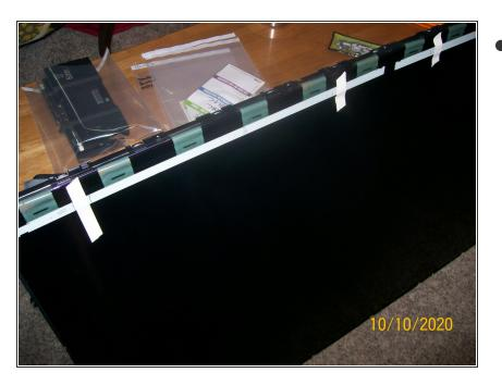
Now you'll need to remove the plastic frame that holds the display and filters in place. A series of "snaps" need to be un-clipped.
