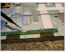
• If you made it this far, congratulations the hard part is done. From now on remember the display now has it's glass panel in place. Be careful if leaning over the display. Un-tape the PCB from the glass and fold them under the frame. The next step is to install the metal bezel that holds the glass panel in place. Easy does it from now on.
