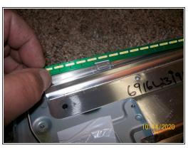
• The tools I used and the strips ready for installation. The fine people at LG make it fool proof to insert the new strips by putting a cutout in the strip and a tab in the frame. REMEMBER to test fit the plug into the connector. One side of my LED had misaligned pin that I had to straighten to get the plug to fit. Very difficult to do in frame.
