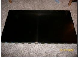
Once the filters are in place, make sure the filters are flat and the snaps secure. Now comes the trickery park. Replacing the glass display panel. If this goes wrong forget about this TV. A new display cost's \$560.00! Lay the display into the frame CENTERED. If you find it's off center DO NOT LIFT ONLY ONE CORNER lift along the whole side.
