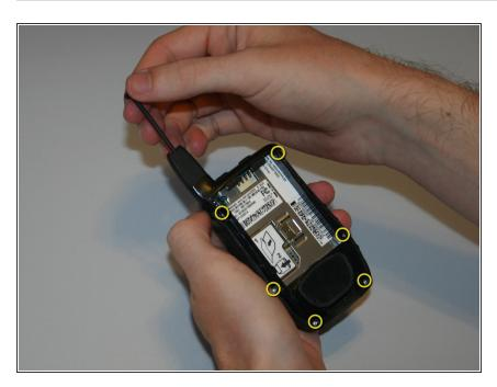
Pull the antenna up to reveal two of the six screws.
