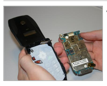
Remove the motherboard from the front half of the phone by gently shaking it loose. It should come out with little to no trouble.
