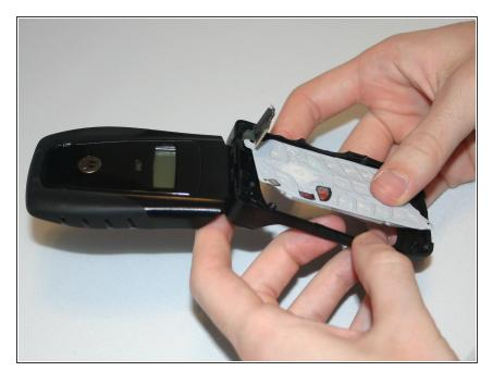
Push lightly from the front of the keypad to remove it.
