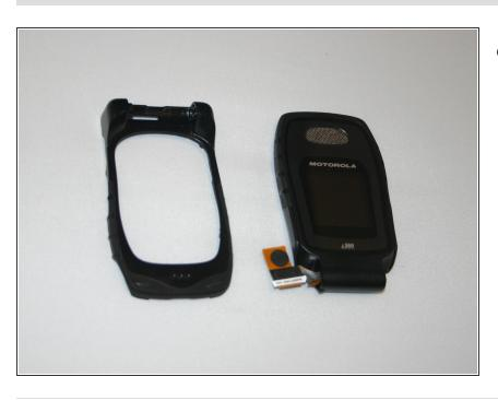
After sliding the ribbon cable through the front frame of the phone, the separated screen and phone frame will appear as shown.
