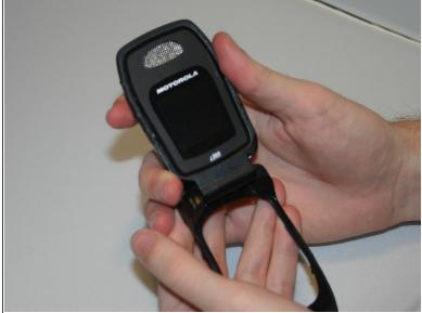
• By applying force, "pop" the screen out of the connecting hinge frame of the phone.
