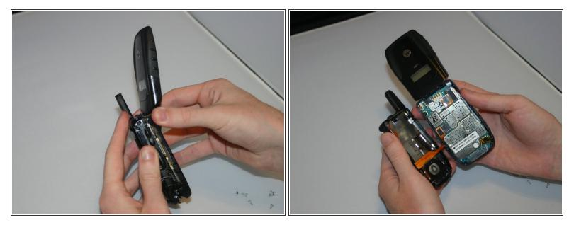
Gently separate the front and back sides of the phone, as shown in the picture.
