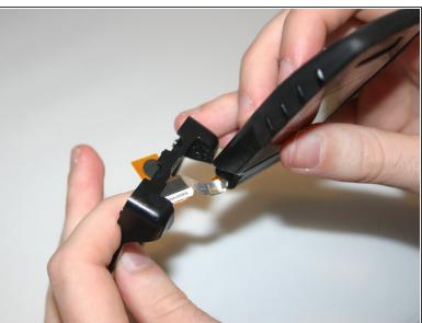
Carefully slide the speaker ribbon cable through the slot in the front frame of the phone.
