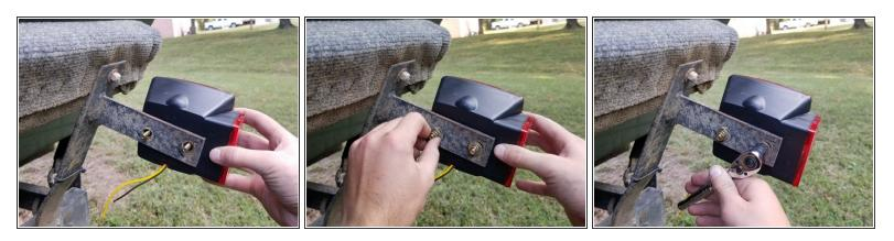
For installing the new light on the mounting bracket on the driver side, repeat steps 9 and 10.
