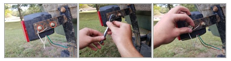
Use a ratchet wrench to remove both hex nuts on the bolts mounting the light to the bracket.
