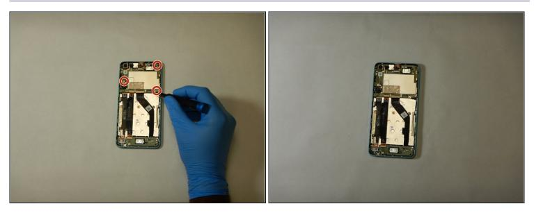
• Remove the three 4.0 mm T5 Torx screws connected to the motherboard.
