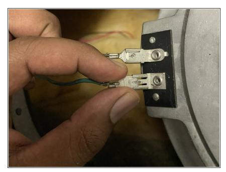
Unlatch the green wire by pulling on the terminal connector and not the wire.
