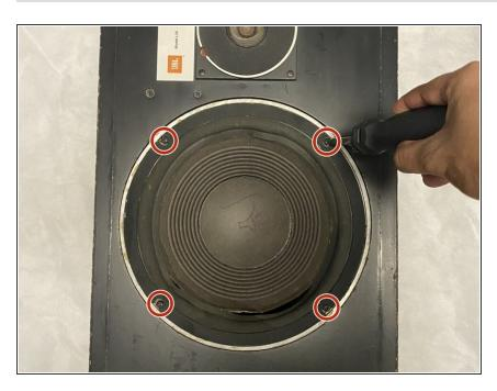
Remove the four 6.4 mm Phillips #2 screws from the front of the speaker.
