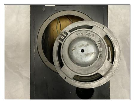
Pull the speaker out of the frame and lay it onto the side.
