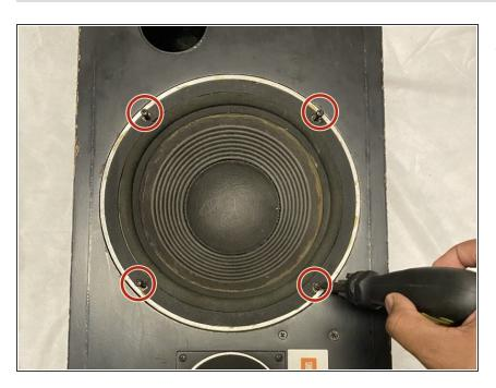
Place the new speaker onto the frame and screw the four 6.4 mm
