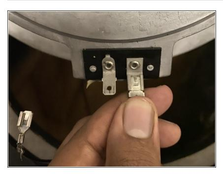
Get your replacement speaker and connect the green wire by pushing the terminal connector onto the tap.
