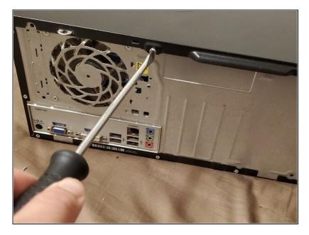
• Remove the 10 mm flathead screw on the back panel with a flathead screwdriver.
