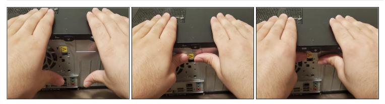
• Slide the side panel back towards the back panel of the computer.
