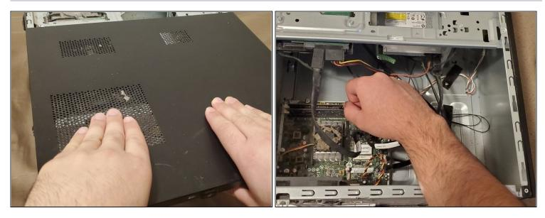
• Continue sliding the panel back until it is about halfway off the computer case, then lift it away from the computer.
