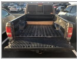
Pull the tailgate latch and lower the tailgate down so that it is open.
