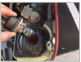
Loosen and remove the taillight plug so that the bulb is exposed.
