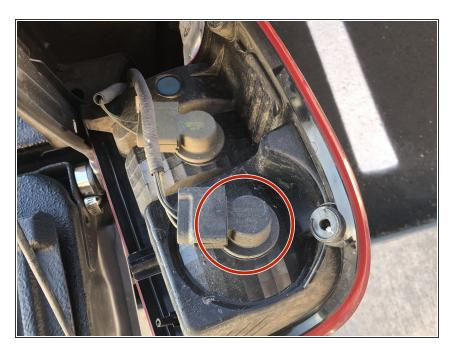
Remove any dirt or dust around the taillight plug so that nothing falls into the lens.
