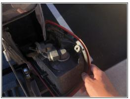
Pull the taillight housing down from the truck so that the wires and plugs are exposed.
