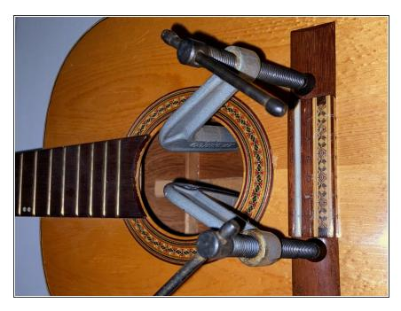
• Use a C-clamp to gently clamp the bridge to the body of the guitar.
