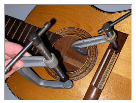
• Remove the clamp after glue has dried.
