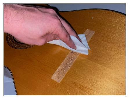
• Carefully remove any excess glue or debris on the body of the guitar from the old bridge.
