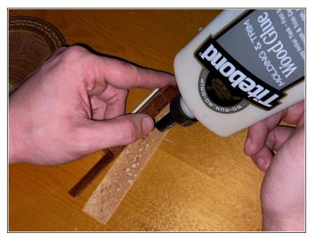
Apply wood glue to the new bridge and attach it to where the old one used to be.
