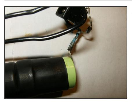
Once the contacts are trimmed to size, the battery is ready for installation into the screwdriver.
