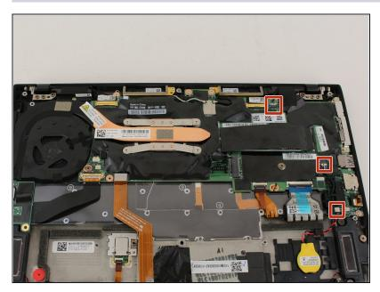
Remove the insert connections by pulling the connector away from the port.
