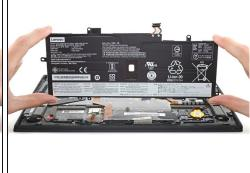
• Lift the battery straight out of its recess and remove it.
