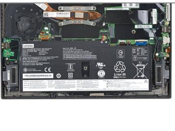
Use a Phillips #0 screwdriver to remove the six 4.9 mm-long screws securing the battery.
