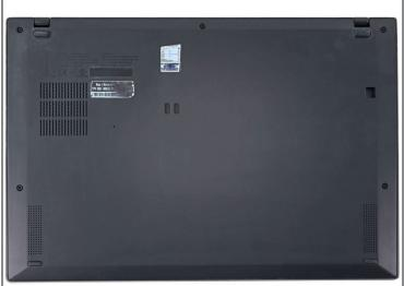
Use a Phillips #1 screwdriver to loosen the five captive screws securing the back cover.
