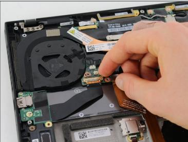
• Remove the connectors with bar latches by lifting up on the small bar behind the port and pulling the circuit ribbon away from the port.
