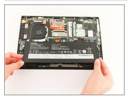
Take out the battery by lifting it from the bottom edge of the laptop, and then pulling away from the motherboard.
