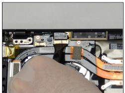
Disconnect the two display cables from the motherboard by lifting the press fit connectors off the board with a spudger.
