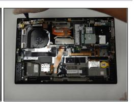
• Using a Phillips #0 screwdriver, remove the six 5 mm screws connecting the display hinges to the device.
