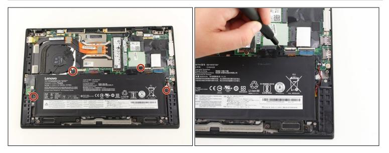
• Use the Phillips #0 screwdriver to remove the four 5 mm screws that secure the battery to the laptop frame.
