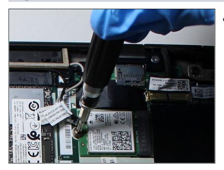
Use a Phillips #0 Screwdriver to unscrew the 3 mm screw holding down the Wifi card.
