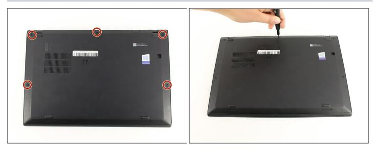
• Use a Phillips #0 screwdriver to unscrew the five screws that secure the back cover to the laptop.
