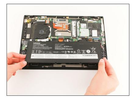
• Take out the battery by lifting it from the bottom edge of the laptop, and then pulling away from the motherboard.
