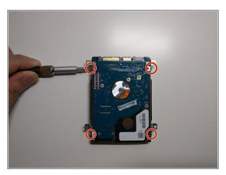
Remove the four screws on the side of the hard drive casing using a Phillips #0 screwdriver.
