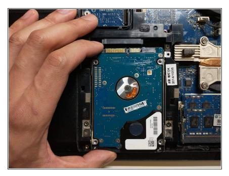
Slide the hard drive out from its slot.
