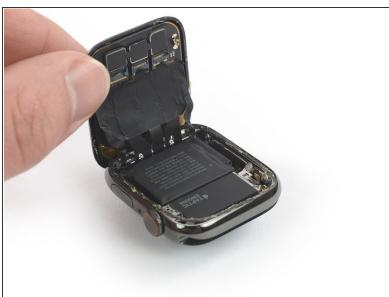
$\begin{tabular}{ll} $\Lambda$ void tensioning the display cables when folding the screen to the back.$
