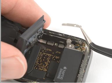
Use a pair of tweezers to remove the metal plate covering the battery connector.
