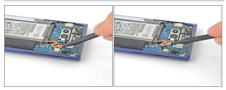
Use the tip of a spudger to disconnect the orange ribbon cable connecting the battery to the motherboard.
