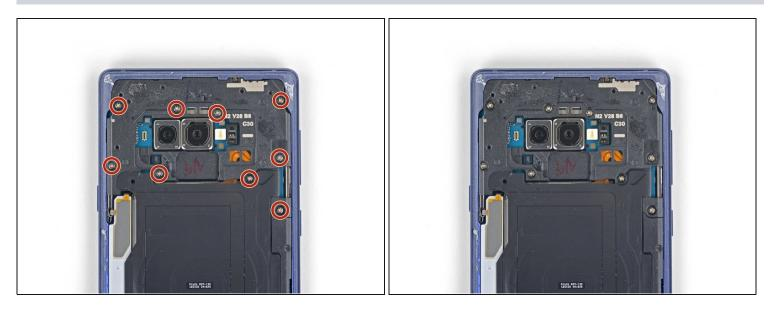
• Use a Phillips screwdriver to remove the nine 4 mm screws securing the upper midframe.
