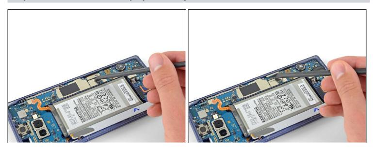
• Use the flat end of a spudger to disconnect the display cable from the motherboard.
