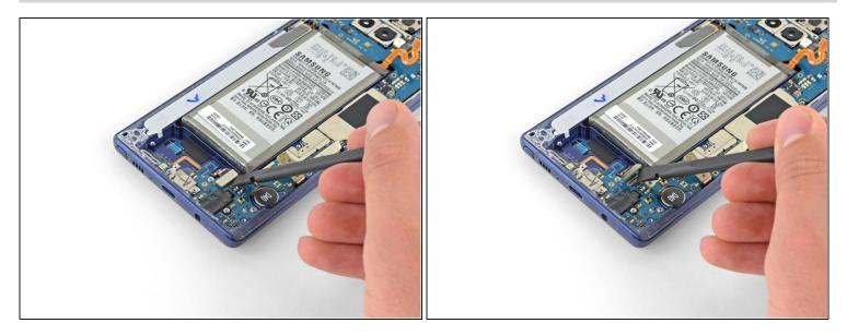
• Use the flat end of a spudger to disconnect the charging assembly from the motherboard.
