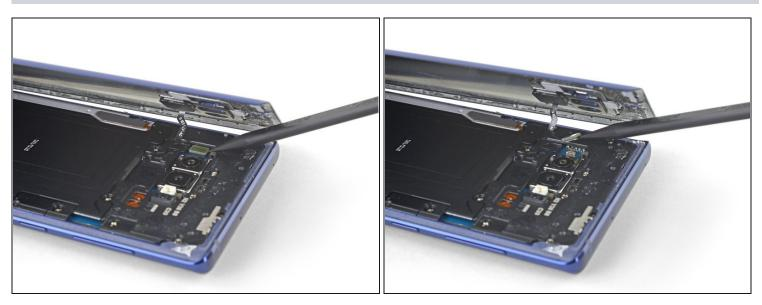
• Use the tip of a spudger to pry the fingerprint sensor ribbon cable up and out of its socket.
