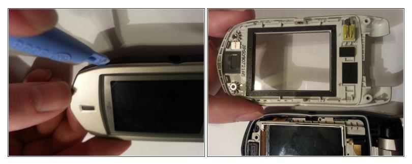
• Use a plastic opening tool to remove the screen cover from the rest of the lid.
