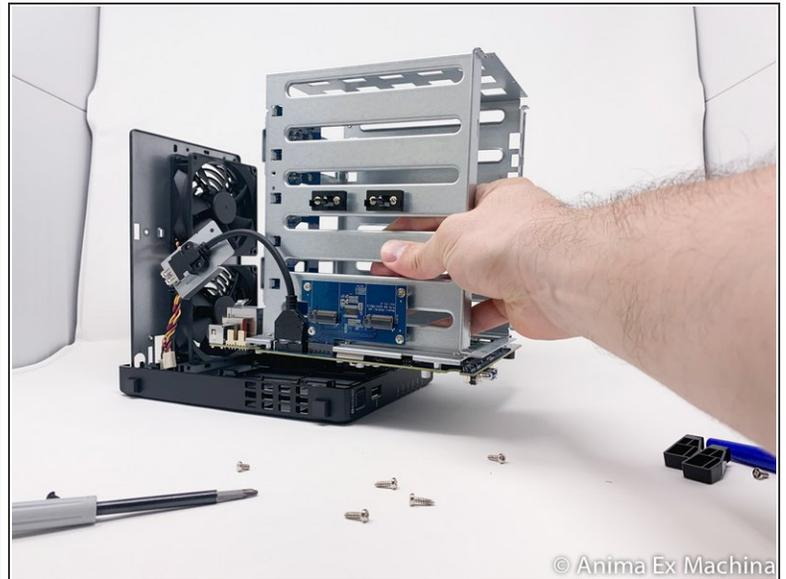
**i** Here, the motherboard is still secure to the disk cage.
