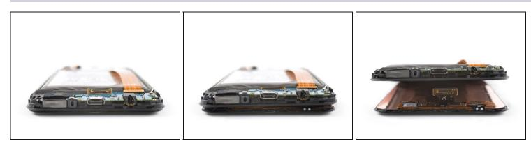
• Thread the display flex cable through the gap in the midframe and remove the display.
