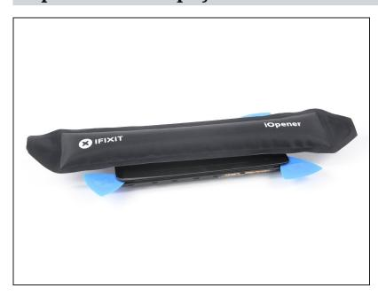
Apply a <u>heated iOpener</u> to the screen to loosen the adhesive underneath its center. Apply the iOpener for at least two minutes.
