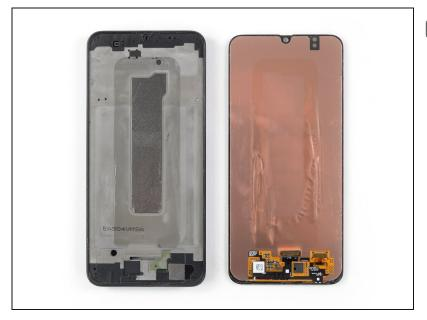
Compare your new replacement part to the original part—you may need to transfer remaining components or remove adhesive backings from the new part before installing.
