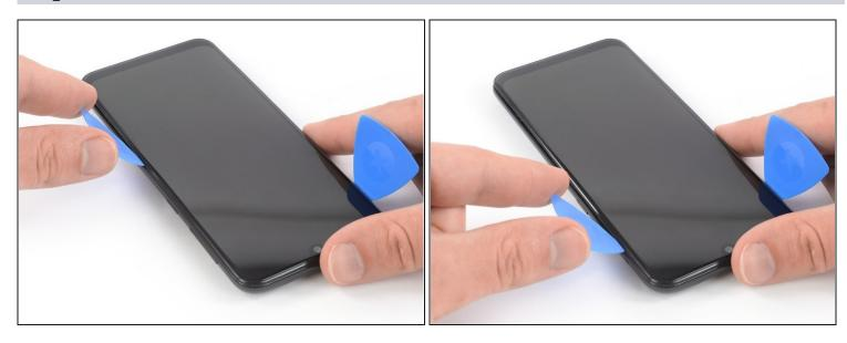
• Slide the opening pick along the right side of the phone to release the plastic clips on the right side of the back cover.
