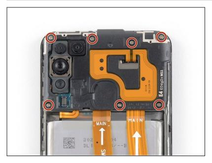
Remove the seven Phillips #00 screws (3.9 mm length).
