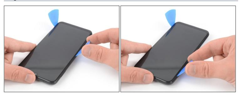
• Slide the opening pick along the left side of the phone to release the plastic clips on the left side of the back cover.
