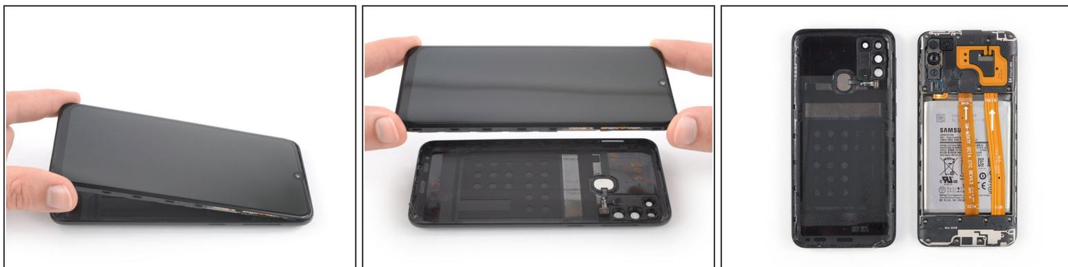
**⚠** The flex cable of the fingerprint sensor is very short and the sensor is likely to disconnect itself during the following removal procedure. Avoid damaging the cable by removing the back cover too quickly.
