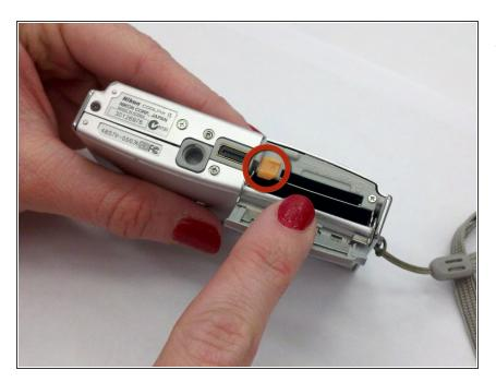
Press orange clip to eject battery (battery not shown).
