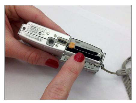
• Following the positive and negative placement signs, slide the new battery into the battery slot (battery not shown).
