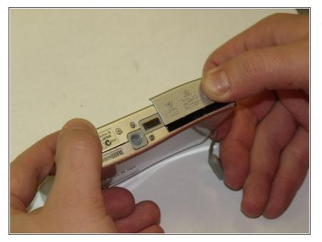
Slide the SD/Battery cover in the reverse direction of the arrow on the SD/Battery cover until it clicks into place.
