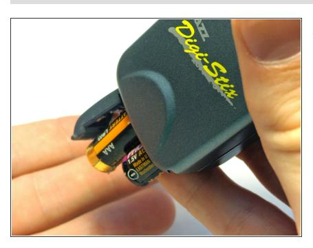
Tilt device so that batteries slide out.
