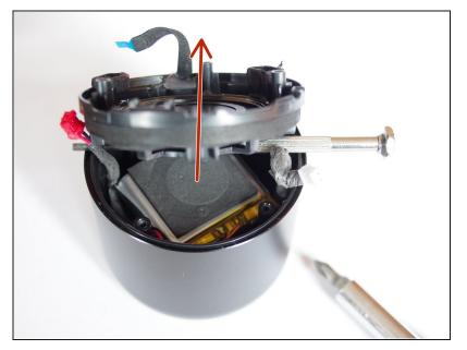
Remove the battery pack carefully by pulling it upward (it is fixed by glue only to the speaker casing).
