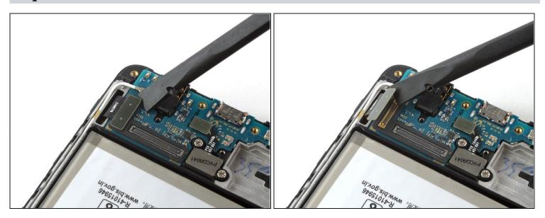
• Use the flat end of a spudger to pry up and disconnect the display flex cable on the bottom of the phone.
