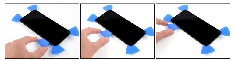
• Insert a fifth opening pick and slide it along the left edge of the phone to cut the remaining adhesive.
