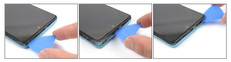
• Slide the opening pick along the top edge to release the top plastic clips.
