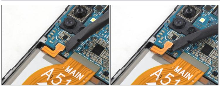
• Use the flat end of a spudger to disconnect the battery by prying the connector straight up from its socket.
