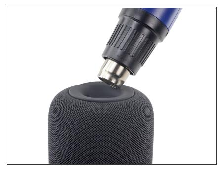
• Using a hair dryer on hot or a heat gun on low, carefully heat up the bottom foot for 1-2 minutes.
