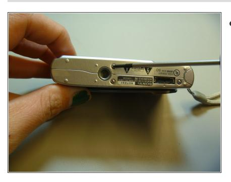
Use screwdriver to remove screws.
