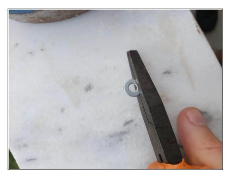
Take an M5 washer and bend a small portion of it at a 90° angle. This will act as a hook that will hold the spring in place, preventing it from slipping.
