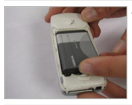
Once the back cover plate is removed, the battery should be exposed. Remove the battery by prying it out. This can be done with your finger-nail or a prying tool.
