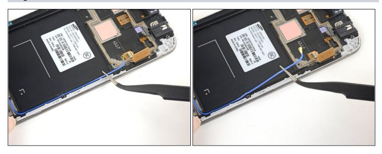
• Use <u>tweezers</u> to lift and de-route the antenna cable from the edge of the case.
