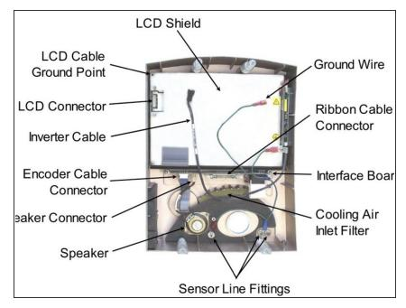
Disconnect the three tubes from the barbed fittings along the bottom of the inside of the front enclosure. Be sure to note where they were connected.
