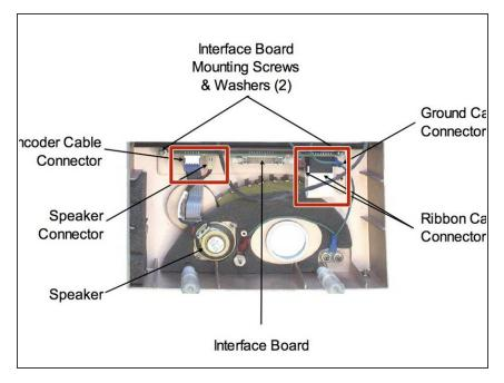
Disconnect the 9 and 2 pin flex cable from the front of the interface board.
