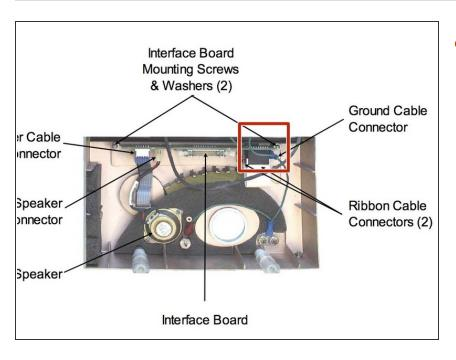
Disconnect the green ground cable from the front of the interface board
