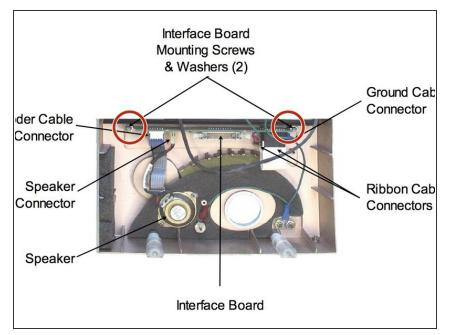
Remove the two 3x8 mm screws and 4mm washers at the two ends of the PC Board with a Phillips Head screwdriver.
