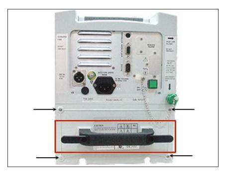
Pull the power pack from the compartment using black handle.
