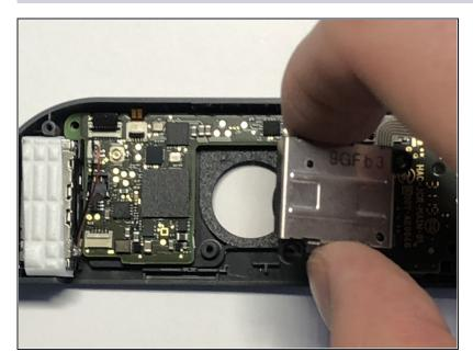
• Gently lift the joystick up and out of its holder.
