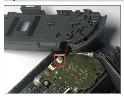
Using a pair of tweezers, gently lift the grey clasp holding down the ribbon cable and slide it out from its connector.
