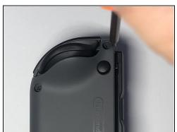
Use a Tri-wing Y00 screwdriver to remove the four 5mm screws holding the back panel in place.
