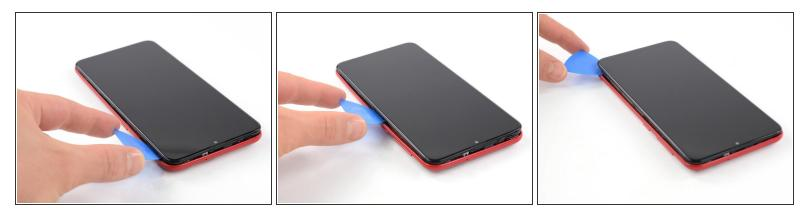
Slide the opening pick from the top left corner to the bottom right corner to release the remaining clips.
