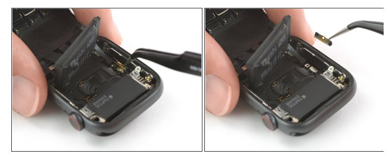
Use a pair of tweezers to remove the metal plate which covers the battery connector.
