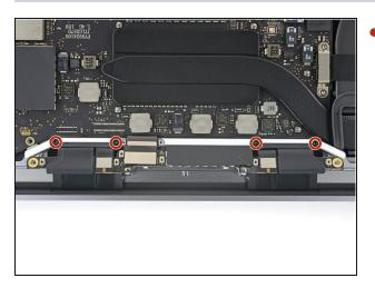
Remove the four 3.9 mm T3 Torx screws securing the spring hinges of the two display cables.
