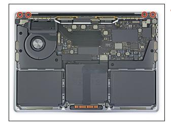
Remove the four 3.3 mm T3 Torx screws securing the plastic covers on top of the display hinges.
