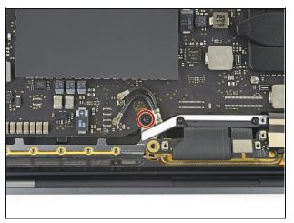
Remove the 3.4 mm T5 Torx screw securing the two antenna coax cables to the main board.
