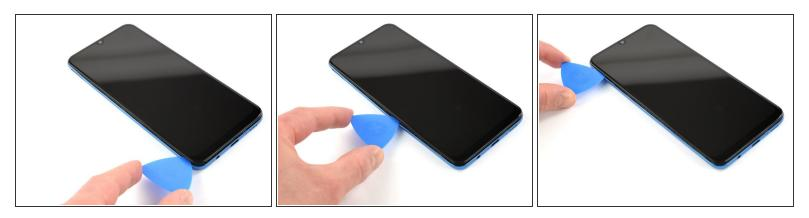
Continue sliding the pick along the left edge of the phone to release the clips.
