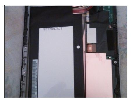
Note battery compartment slightly larger than battery. 1/8" reveal on left side if off after top of battery shifted.
