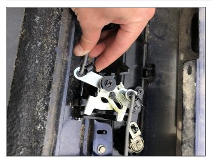
• Insert cable back into socket and press rubber lock onto cable.
