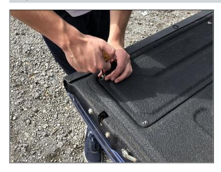
Put panel back into place and screw in using your torx -T25 screwdriver.
