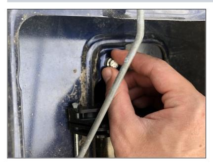
• Hand twist in bolts; then tighten with wrench.
