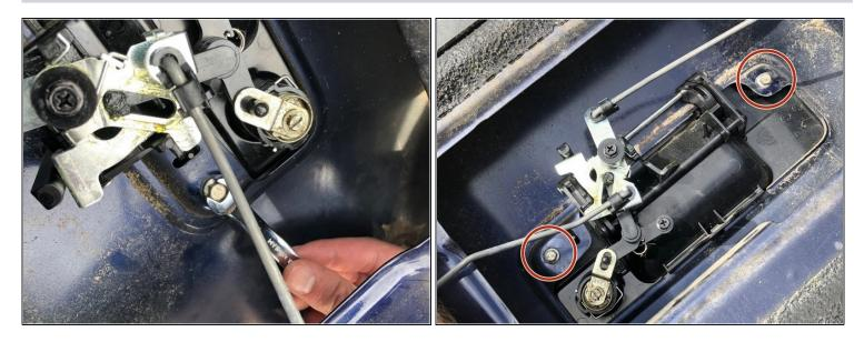
• Use your 5/16th-in. wrench to turn bolt counter clockwise and remove the bolts (18.5mm).
