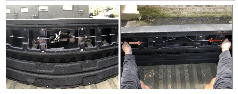
• Pull off the panel and then pull cables inward, causing tailgate to release and go down.
