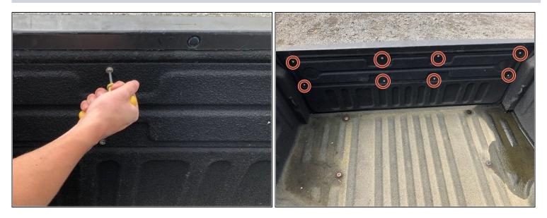
Remove the Torx-head screws (23.2mm) on the inside panel of the tailgate, using the torx T25 screwdriver.
