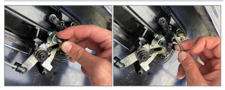
• Remove rubber pieces from cable and pull cable from insert.
