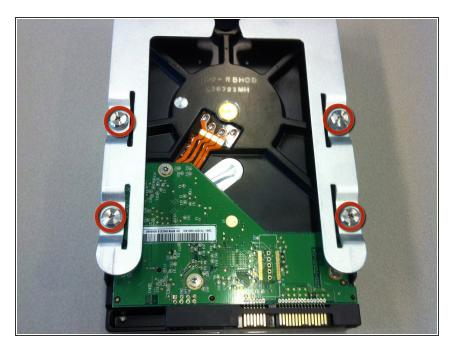
Remove your new hard drive from its packaging and use a phillips head screw drive to attach it to the bracket. Use the screws that are already included on the bracket.
