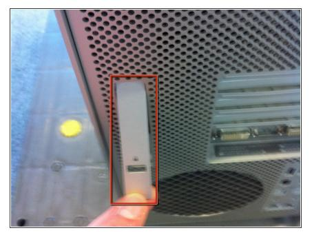
• Open the Case Shut down your Mac Pro, give it a few minutes to cool off, and unplug all the wires and cables. Locate the latch on the back of the case and pull it out. The latch lifts out very easily and stops after an inch or two — do not try to force it any farther.
