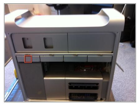
• With the Mac Pro's case now open, locate the four hard drive bays in the top half of the case.
