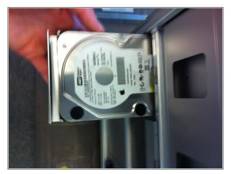
Each bay has a number stamped on it, and they go in order from left to right. Bay #1 should contain the stock hard drive that was installed by Apple. Gently remove the bracket from the next empty hard drive bay
