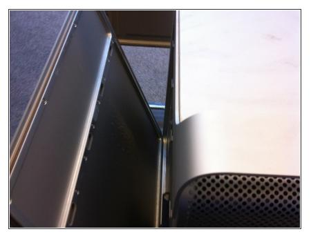
Opening this latch releases the side panel of your Mac Pro, which you should now be able to easily lift away from the case. Take it off and put it in a safe place
