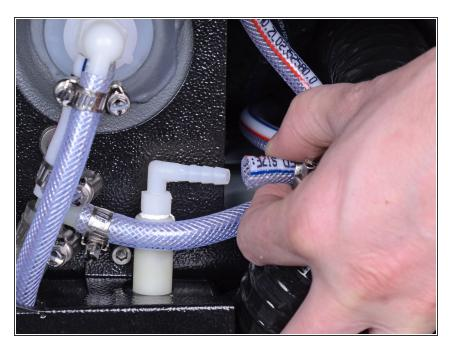
Pull the check valve hose straight off of its hose barb to remove it.
