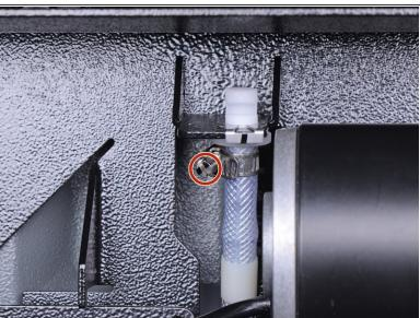
Use a flathead screwdriver to loosen the hose clamps at each end of the check valve hose.
