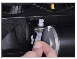
Use an angled pick or your fingers to pull the clamp securing the check valve hose nozzle straight out and off of its bracket.
