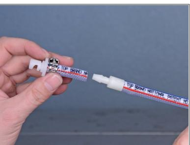
Pull the shorter hose straight off of the check valve to remove it.
