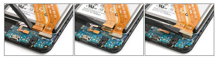
• Use the flat end of a spudger to pry up and disconnect the charging port and display flex cables from the daughterboard.
